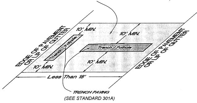
NOTE: \* IF THERE ARE 2 OR MORE TRENCHES WITHIN 300 FEET OF THE STREET, THE SLURRY SEAL SHALL APPLY CONTINUOUSLY TO COVER ALL TRENCHES.
