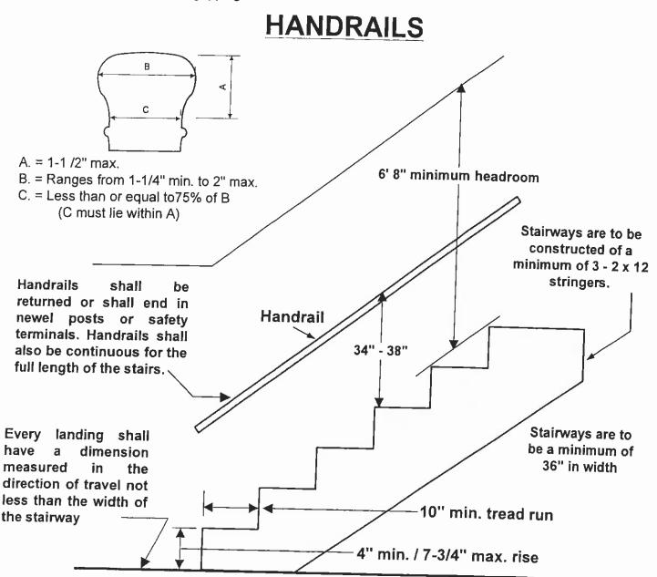
The largest tread run & the largest riser height within any flight of stairs, may not exceed the smallest (respectively) by more than 3/8".
