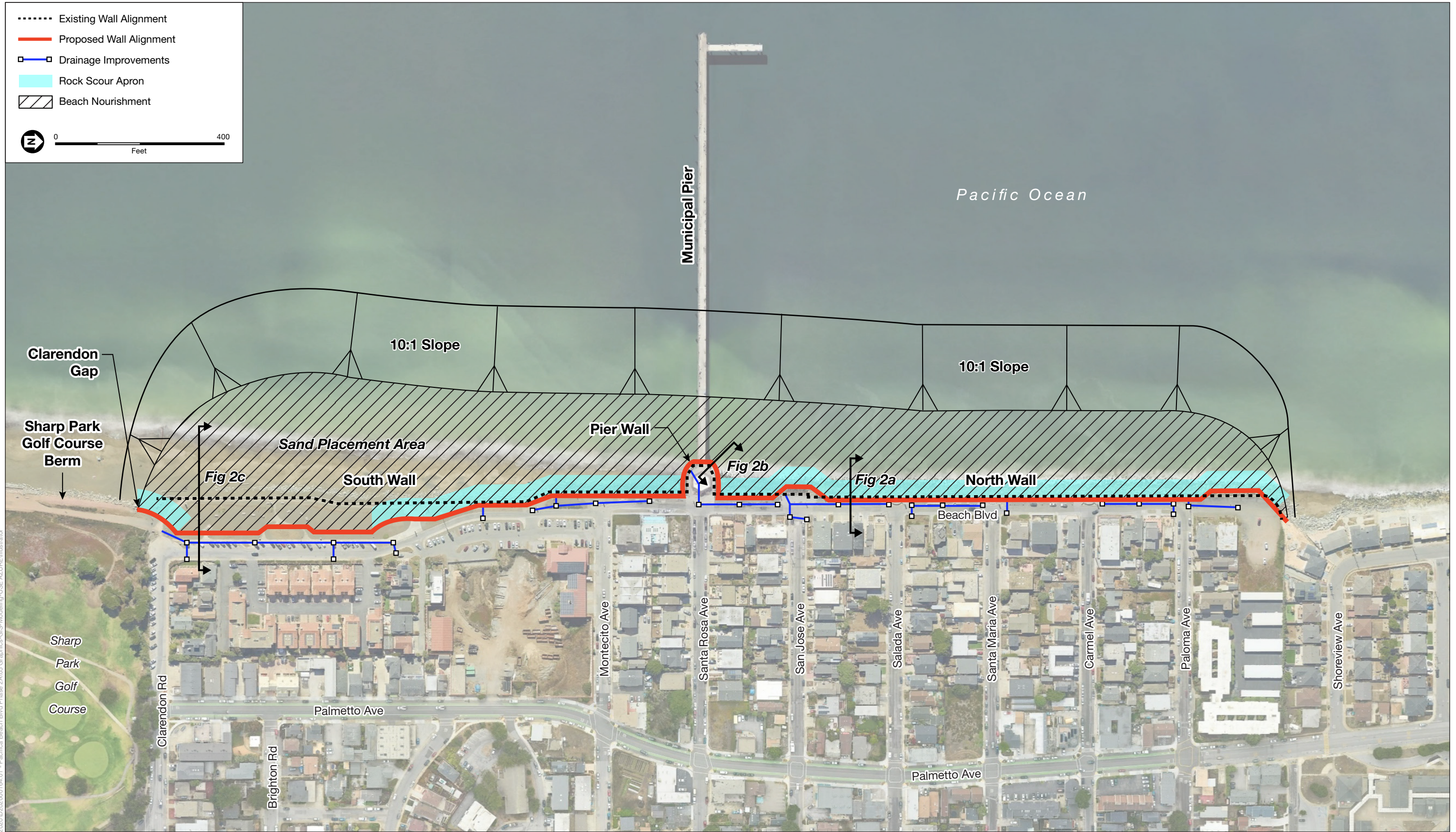
Figure 2 Existing and Proposed Seawall Alignment, Rock Scour Apron, and Beach Nourishment Area
