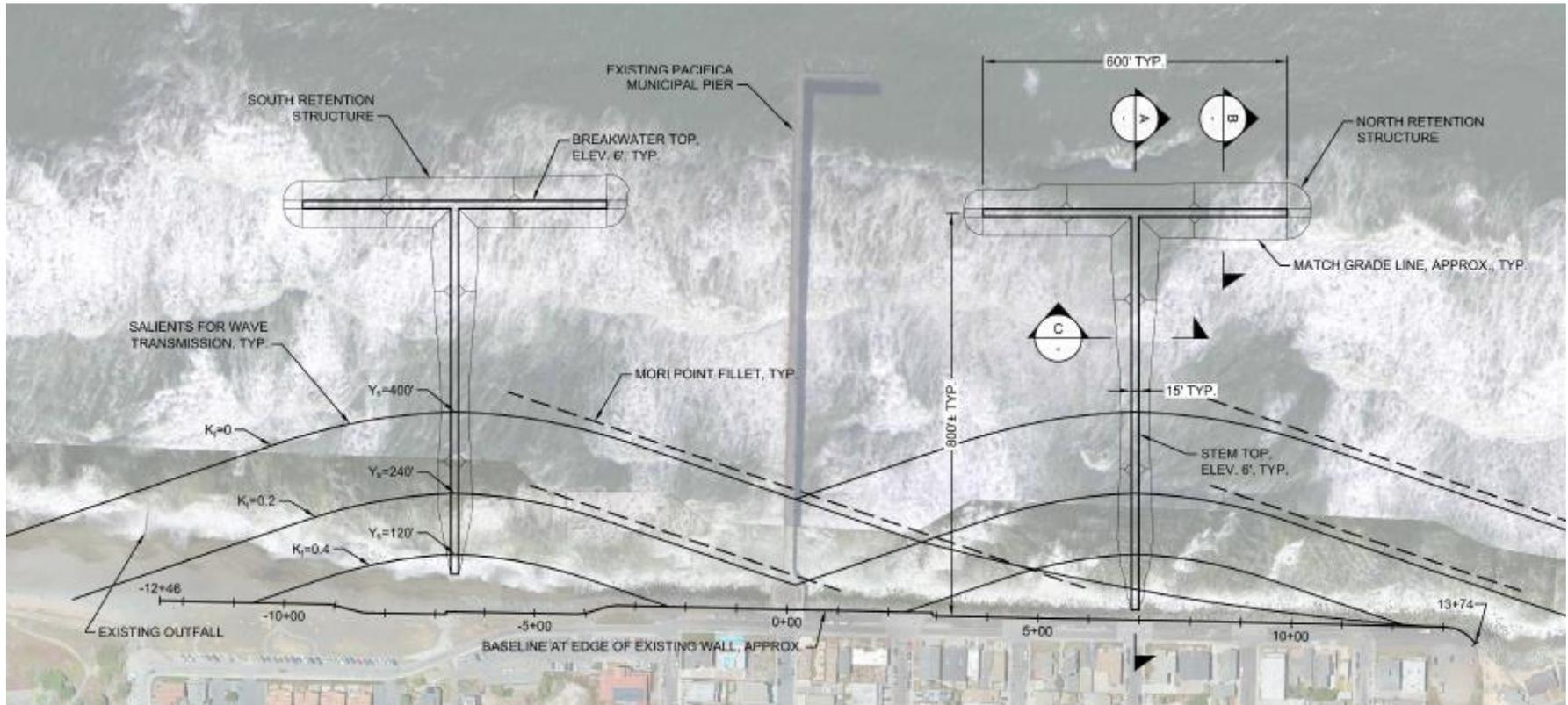
**Figure 3-5 Low-crested Breakwaters, Sand Retention Alternative<sup>4</sup>**
