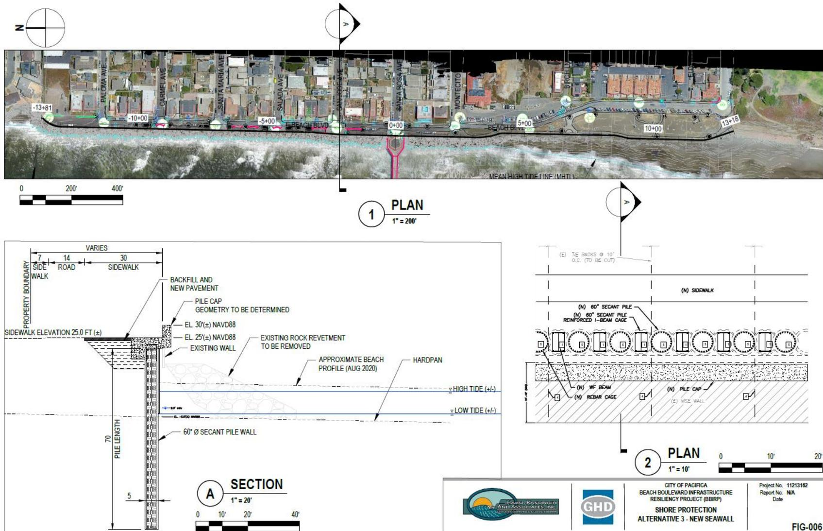
Figure 3-2 Seawall Alternative
