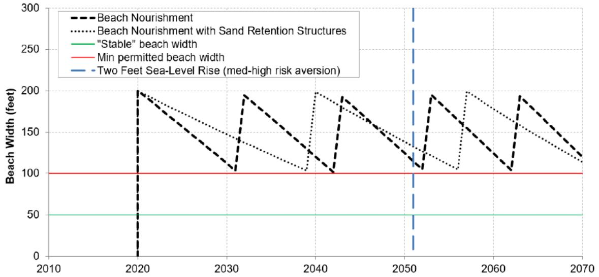
**Figure 3-4 Beach Nourishment Timeline with and without Sand Retention**
