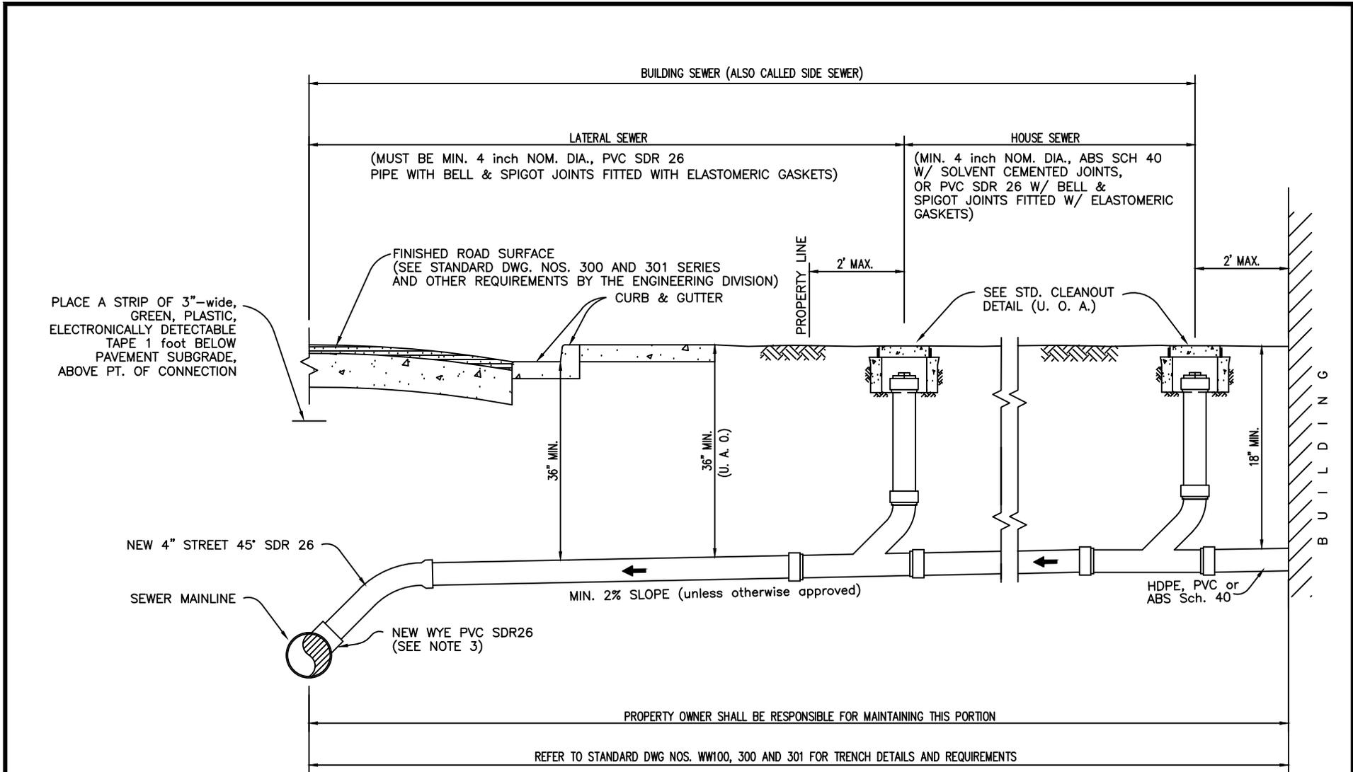
PLACE A STRIP OF 3"-wide, GREEN, PLASTIC, ELECTRONICALLY DETECTABLE TAPE 1 foot BELOW PAVEMENT SUBGRADE, ABOVE PT. OF CONNECTION
