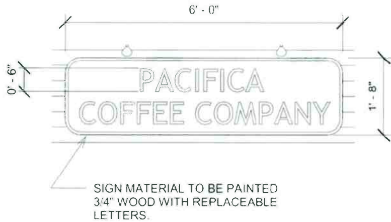
2 FLUSH WALL SIGN DETAIL 1/2" = 1'-0"
