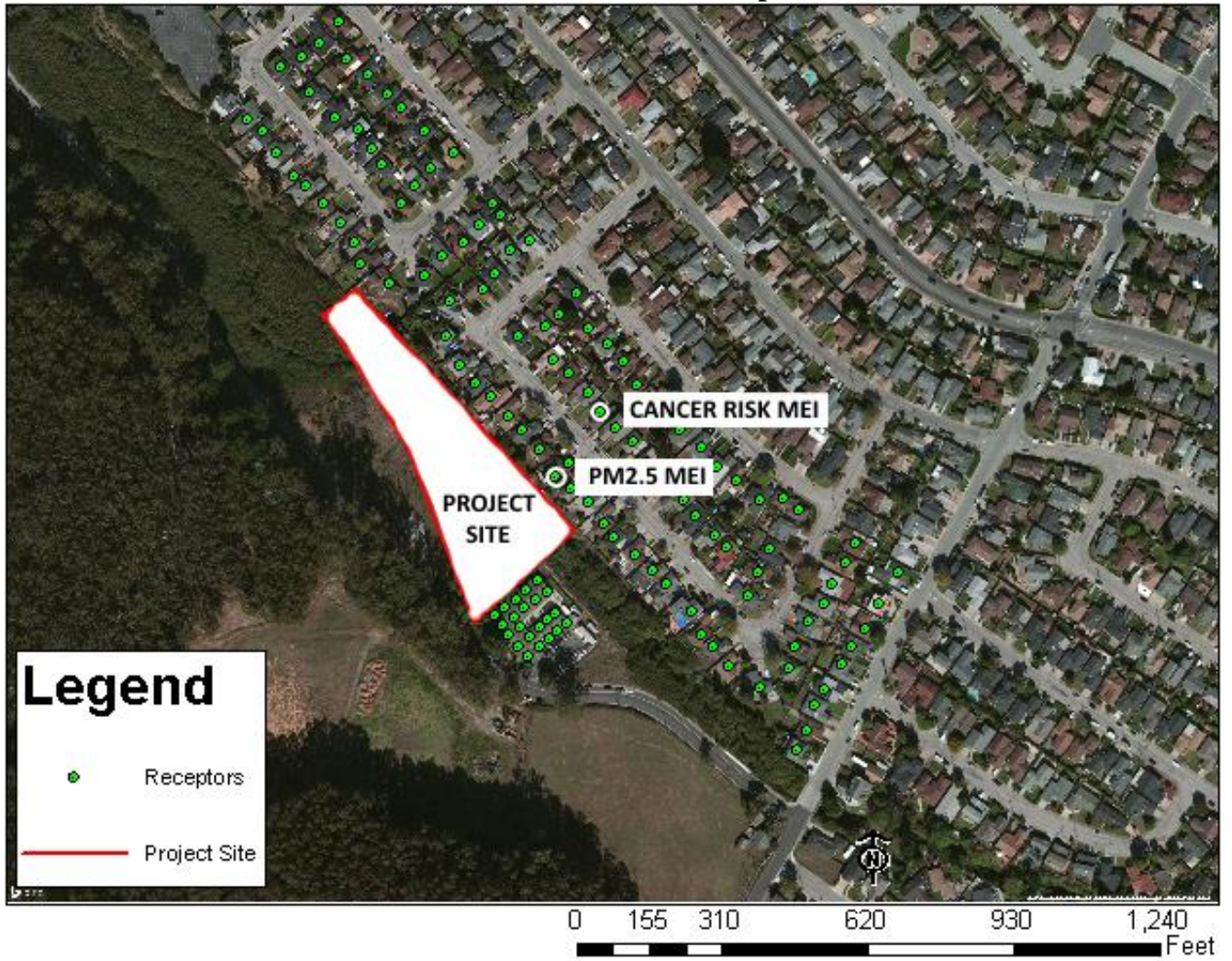
Figure 1. Project Construction Site and Locations of Off-Site Sensitive Receptors and Maximum TAC and PM 2.5 Impacts
